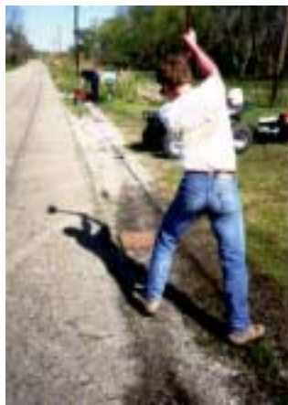
Figure 3. Seismic Energy Sources: Sledge Hammer (left) and drop weight (right) (Louisiana)
