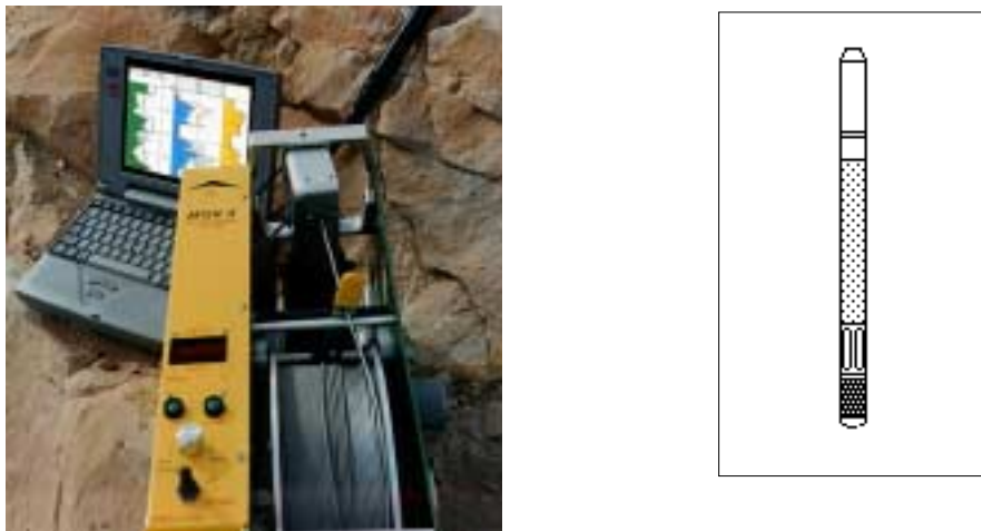
Figure 1. Left hand photograph is a logging winch, cable, and laptop. The right hand drawing is a fluid probe 21-in long by 1.5-in diameter (courtesy Layne-Christiansen Colog, Golden CO).
